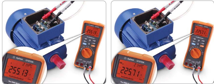
Comparison of voltage output from industrial motor VFD without and with Low Pass Filter functionality.
